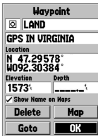
Figure 5. Waypoint Screen - Location is given in decimal degrees yours should look identical to this.
